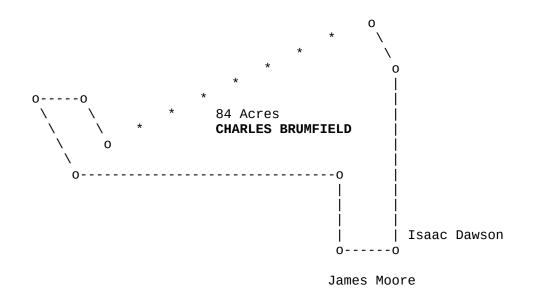
Plotted by a scale of 100 poles in an inch
